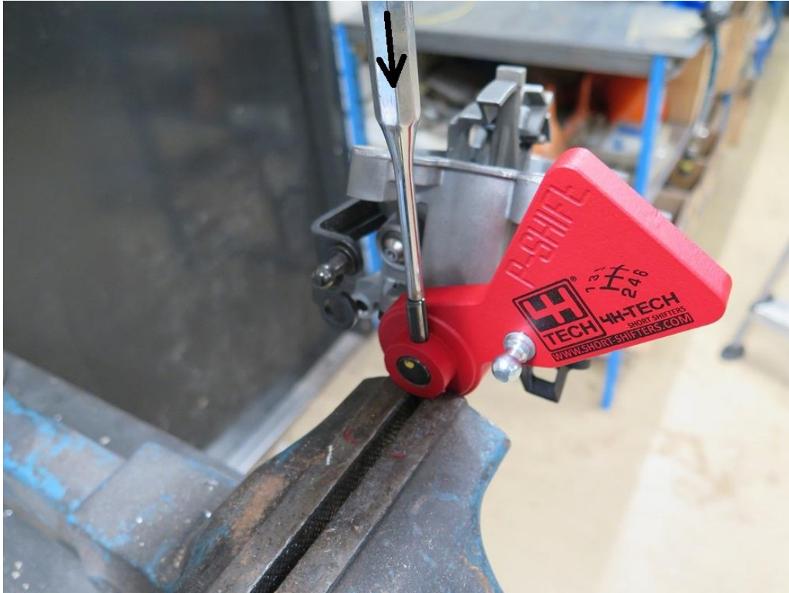
Use the old pin to fit the new shifter on the shaft. (use cotter pin driver tool )
