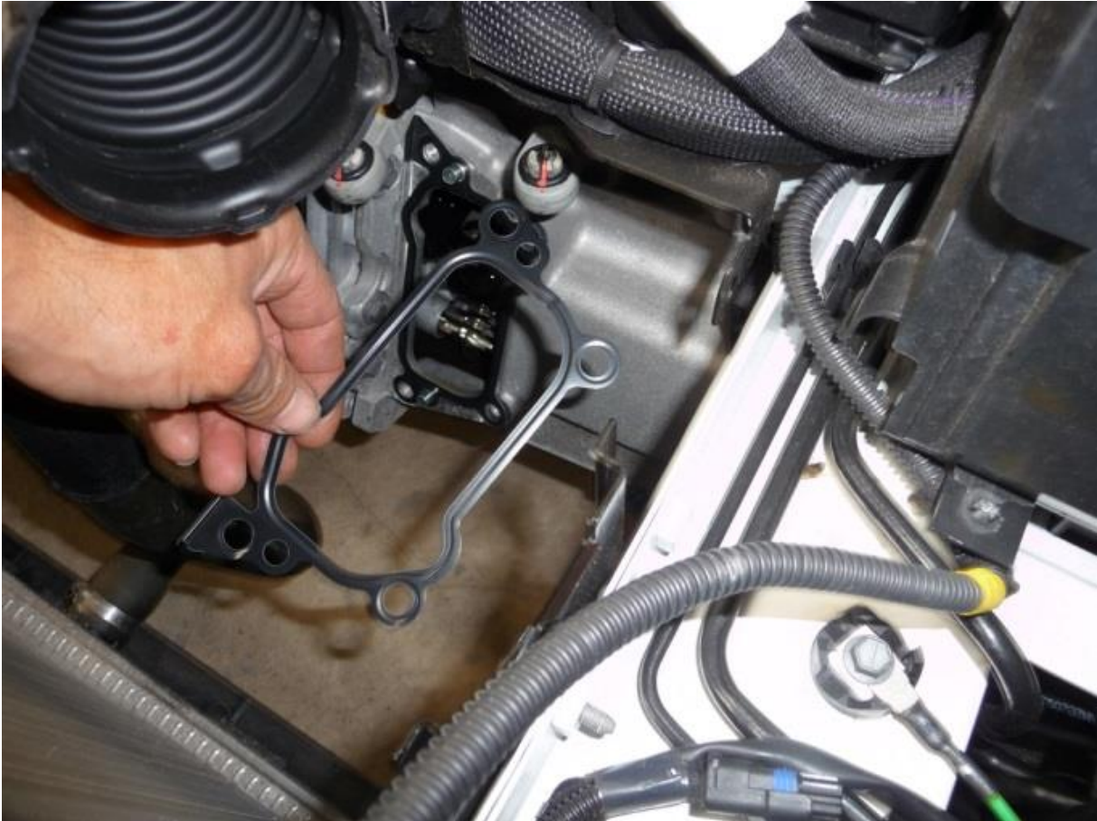
Remove the old seal, and fit a new metal seal. (part number: 245071 at Peugeot or Citroën) Bolt shift unit in place.
