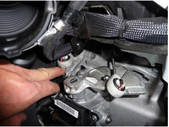
Remove the 2 shift cable ends from the ball heads with a plier.
