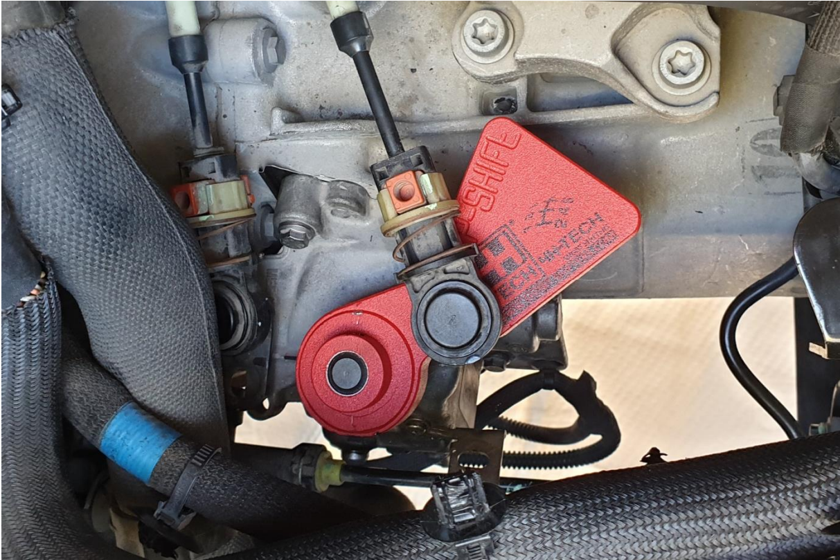
Remove the old seal, and fit a new metal seal. (part number: 245071 at Peugeot or Citroën) Bolt shift unit in place.
