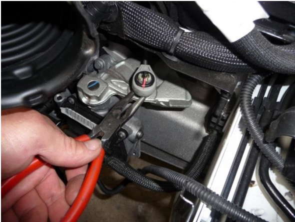
Remove the 2 shift cable ends from the ball heads with a plier.
